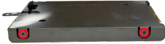
Fig. 4 Unscrewing the hard disk drive shield screws
